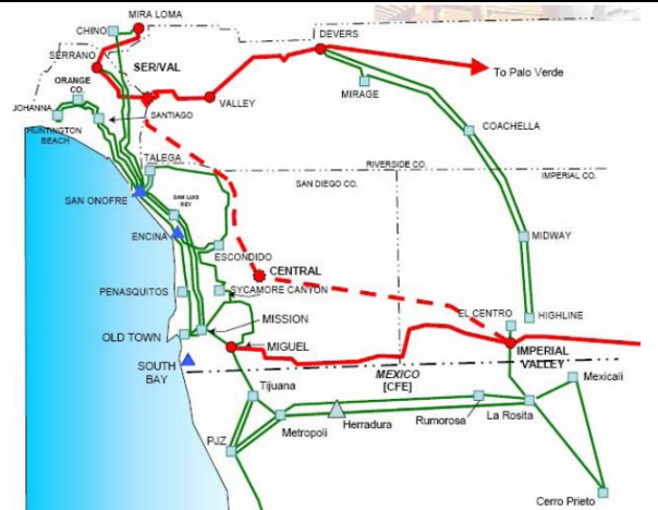
Figure B1. This concept map showing the Sunrise Powerlink ultimately interconnecting with the Los Angeles area transmission grid was submitted by SDG&E in its March 6, 2006 letter to the U.S. DOE requesting “national interest electric transmission corridor” status for the transmission line.
